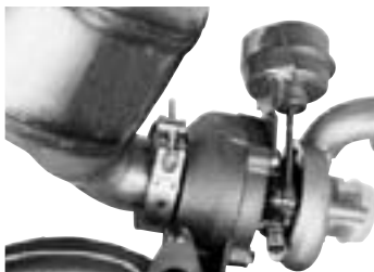
Automobielsector: verbinding turbolader/katalysator
