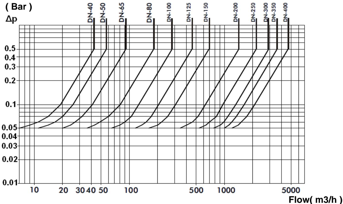
**FLOW COEFFICIENT KV ( in m3/h ) :**
